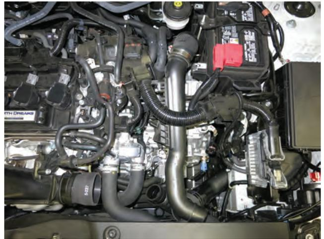
n. Begin removal of the charge pipe from the engine bay by rotating the pipe counter-clockwise. Refer to image above for the desired orientation.
