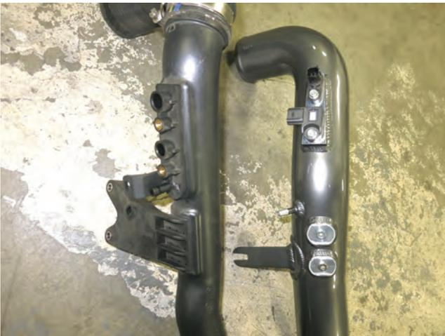
c. Using the stock hardware and an 8mm socket, transfer the MAP and IAT sensors from the stock charge pipe to the AEM charge pipe.
