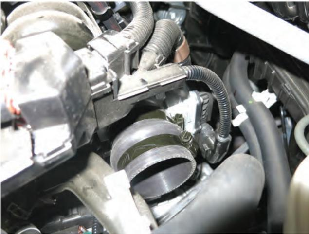
e. Install the hump hose coupler onto the throttle body, with the supplied hose clamps. Tighten the hose clamp on the throttle body side to 30 in-lbs.
