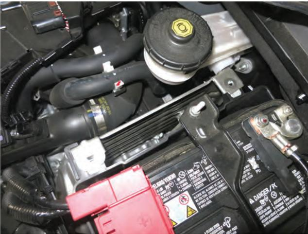
g. Use a 10mm socket to remove the (2) M6 bolts fastening the battery heat shield. Remove the heat shield. Do not discard these components.
