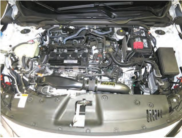
STOCK CHARGE PIPE INSTALLED
