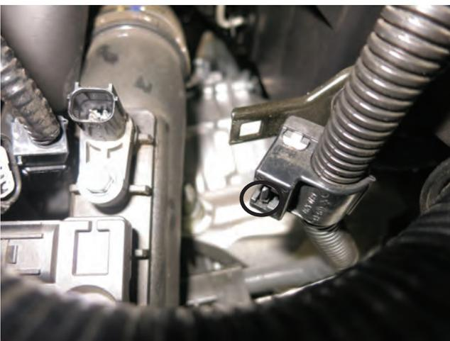
i. Pull on the small tab, circled above, then pull the harness from its mounting bracket.
