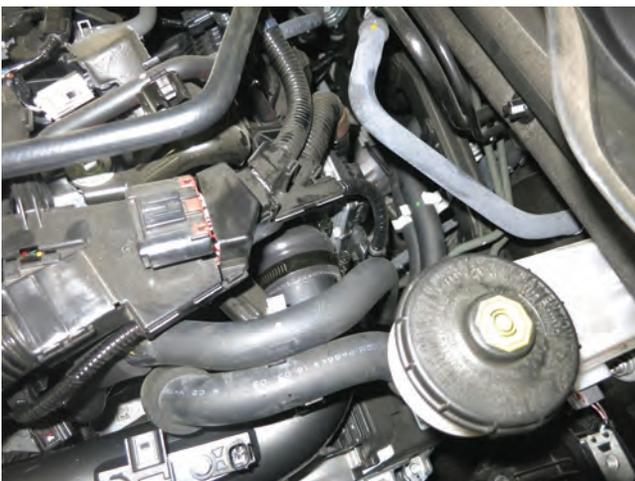
i. Once the charge pipe is in its proper location, insert the upper end into the throttle body coupler. Do not tighten the hose clamp yet. You may reattach the heater hoses into their clips at this time.
