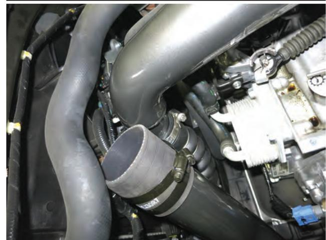
j. Insert the lower end of the pipe into the intercooler hose. It may help to spray the end of the pipe with soapy water. Alternatively, you can heat the hose end with a heat gun or blow dryer. Do not tighten the hose clamp yet.
