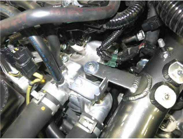
k. Adjust the charge pipe for best fitment. Once you are satisfied, fasten the mounting bracket to the rubber mount with the supplied washer and nut. Also, tighten the hose clamps at the throttle body coupler and inter-cooler hose to 30 in-lbs. You may also remove the tape applied in steps 3a and b at this time.
