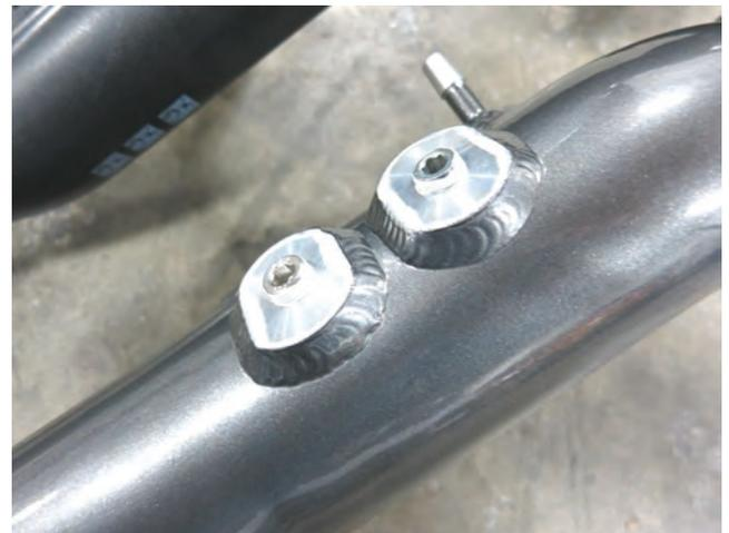
d. If you will not be installing AEM's water/methanol injection kit, thread the supplied 1/8" NPT plugs into the water/methanol injection bungs. Be sure to wrap the threads in Teflon tape beforehand to prevent any boost/vacuum leaks.
