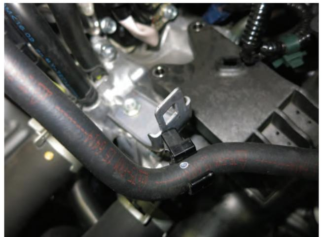
j. Pinch the tabs on the plastic clip holding the vacuum hose you disconnected in step 2d, then pull the clip from the mounting bracket. Move the hose aside.
