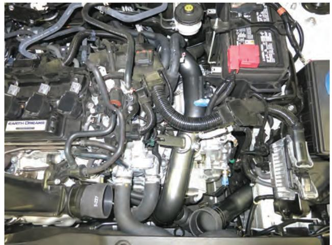
h. Rotate the pipe counter-clockwise as you push it towards the rear of the vehicle. Lower the bottom end of the pipe past the radiator shroud and radiator hose.
