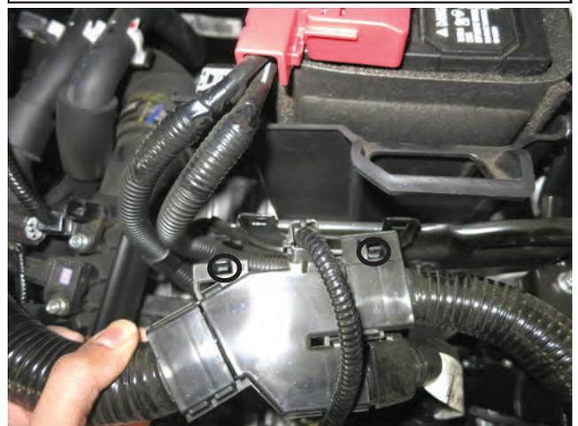
h. Pull on the (2) small tabs, circled above, then pull the engine harness from its mounting bracket.
